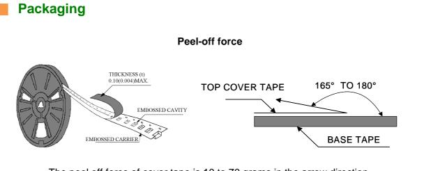
The peel off force of cover tape is 10 to 70 grams in the arrow direction.
