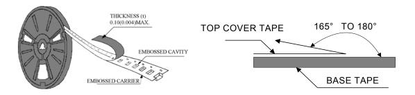
The peel off force of cover tape is 10 to 70 grams in the arrow direction.
