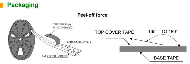
The peel off force of cover tape is 10 to 70 grams in the arrow direction.
