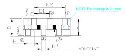
A: 27.0 ± 0.5 mm B: 11.0 ± 0.5 mm C: 8.00 Max. mm D: 2.45 ± 0.10 mm E1: 9.00 ± 0.25 mm E2: 18.0 ± 0.25 mm F1: 6.0 Typ. mm F2: 3.0 Typ. mm G: 10.5 ± 0.20 mm H: 3.6 ± 0.10 mm
