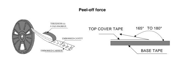
The peel off force of cover tape is 10 to 70 grams in the arrow direction.
